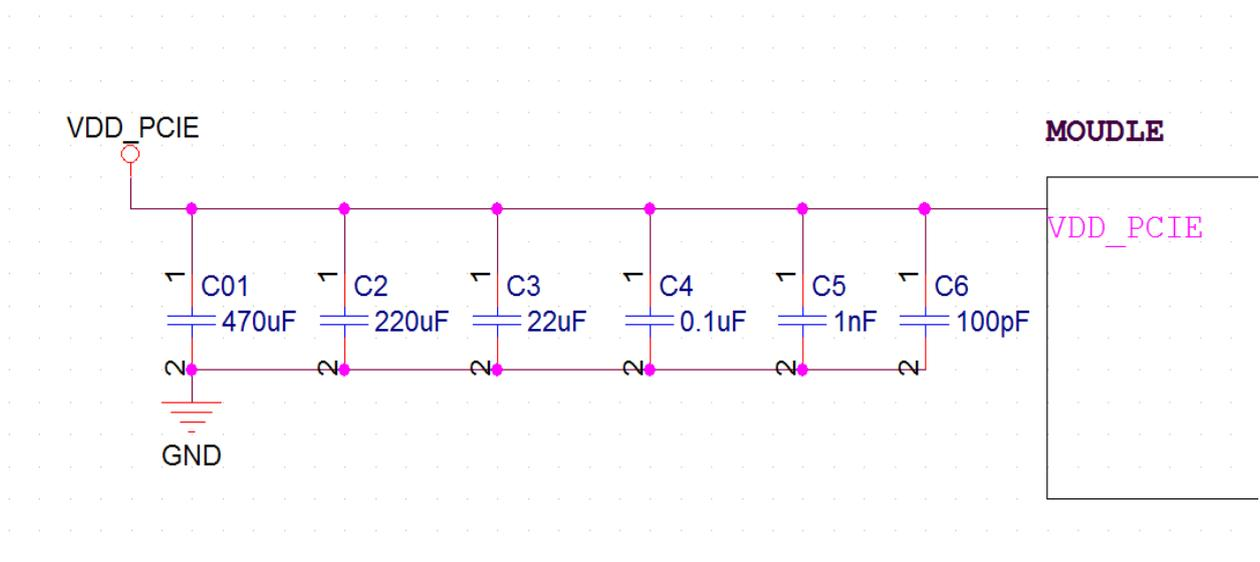
Figure 3 Power Supply Reference Circuit
