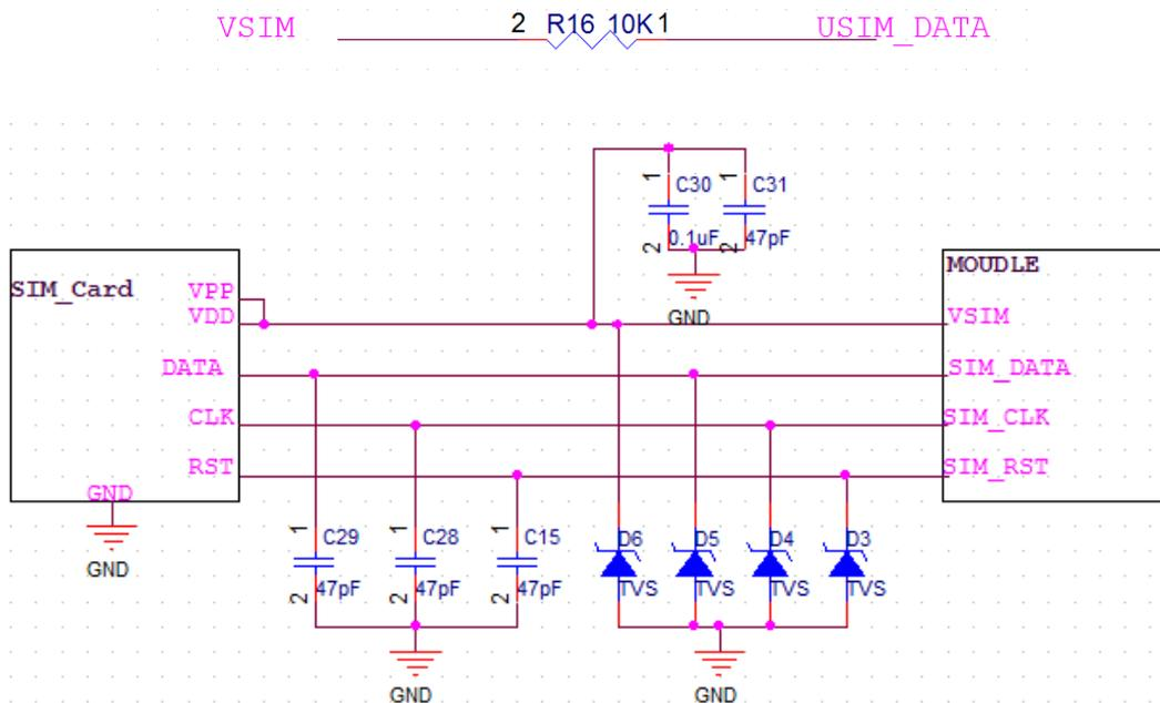
Figure 5 SIM Reference Circuit
