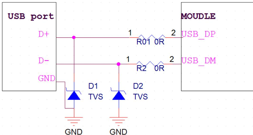
Figure 4 USB Reference Circuit
