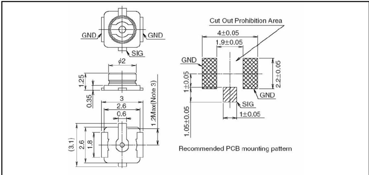
**Figure 4** Dimensions of the antenna connector
